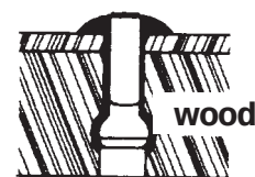
GROOVED RIVET Grooves improve holding strength
