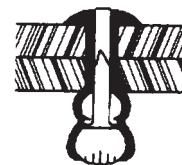
MULTI-GRIP PLUG One rivet does a number of grip ranges
